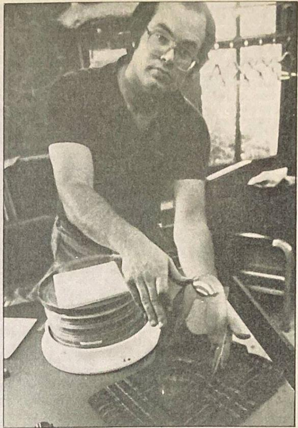
*Rich Schmidt holds the crown glass element of the 12-inch objective when the lens assembly had to be taken apart to re-glue the spacers between the elements.*
